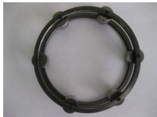
Fig. 3 Cage with rollers
