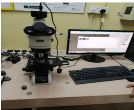
Fig.2 The SHZ10 Stereomicroscope that was used to observe the microstructure and the types of pores in Al 2 O 3 foam.
