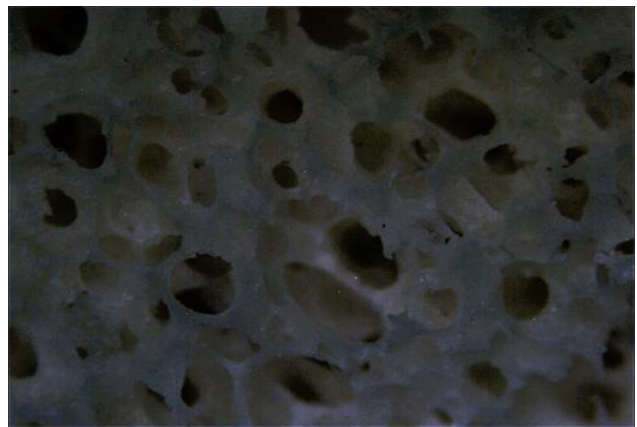
Fig. 8 The microstructure for the Al 2 O 3 foam using with 70 wt% of Al 2 O 3 composition using distilled water as the solvent
