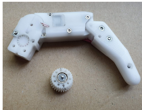
Fig. 11. Manufactured pin and internal gears of the cycloidal reducer assembly.
