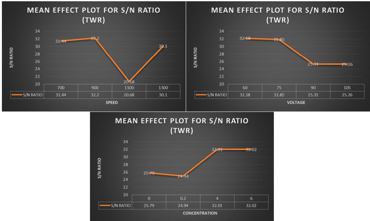
Fig.3b. Main effect plot of mean of S/N ratio for TWR in relation with Speed, Voltage and Concentration
