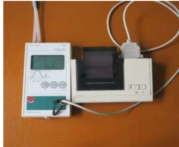
Fig. 3. PulsoTest instrument (Germany) for recording of oscillograms of cow machine milking [1, 2]
