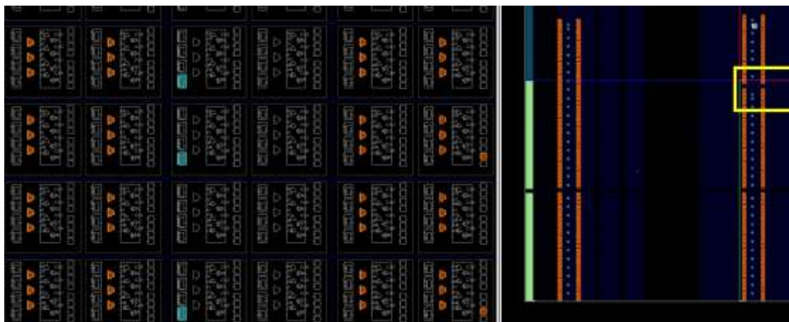
Fig.6. 8-bit Macro placement on the FPGA fabric
