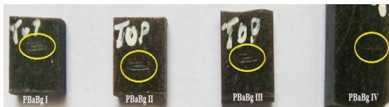
Figure 3. Scratched specimen surface of PBaBg hybrid composites.
