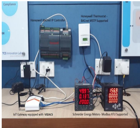
Fig.3. Laboratory Setup - Sensors Connected to IoT Gateway
