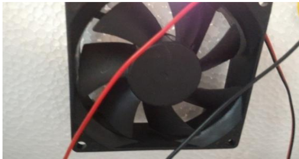
Figure 12b: Temperature sensor output values below threshold level of 420C, cooling fan is in OFF condition
