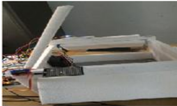
Figure 15b: Rain shield is opened as moisture in the soil is not sufficient.
