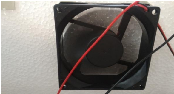
Figure 13b: Temperature sensor output values above threshold level of 420C, cooling fan is in ON condition
