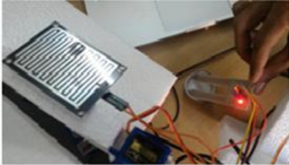
Figure 15a: Rain sensor with soil moisture sensor
