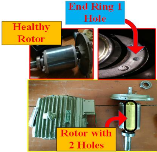
Fig.3. Fault exhibits used in experimental verification
