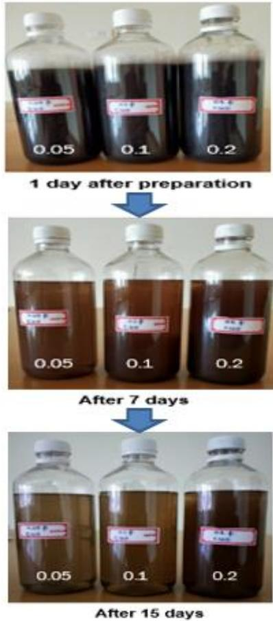
**Fig. 3. Stability check for CuO-DW nanofluid by observation.**
