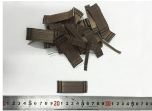
Fig 2: Photograph of double hooked-end steel fibers [34].
