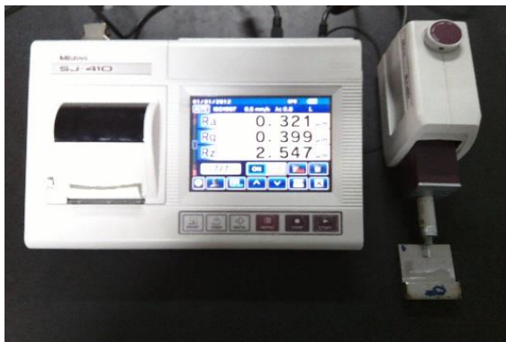
. Fig. 1. Setup for roughness measurement
