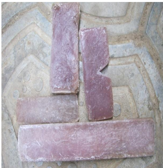
Plate 1: Some sample of cast polyester resin specimens
