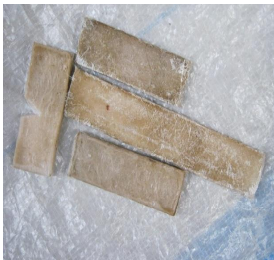
Plate 2: Some samples of cast MKO resin specimens
