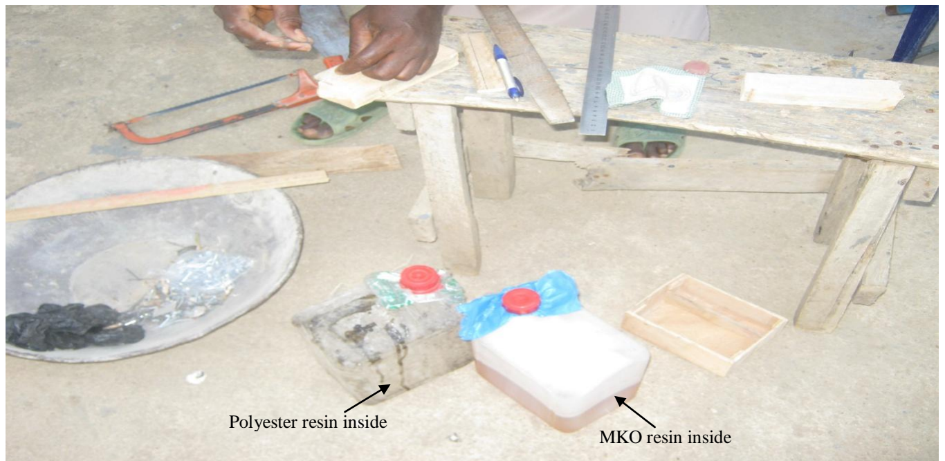
Plate 4: Production of specimens from both MKO and Polyester resins in progress
