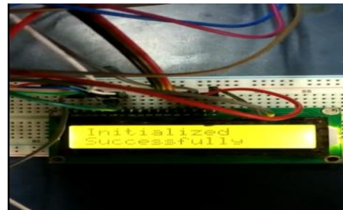
Figure 4: The successful initialization of the system is displayed in the LCD
