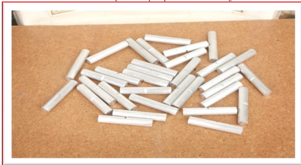
Plate IV: Some of the produced impact specimens before cleaning them
