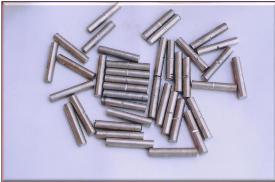
Plate IV: Some of the produced impact specimens before cleaning them
