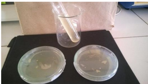
Fig. 7. Revived bacterial colonies from concrete sample
