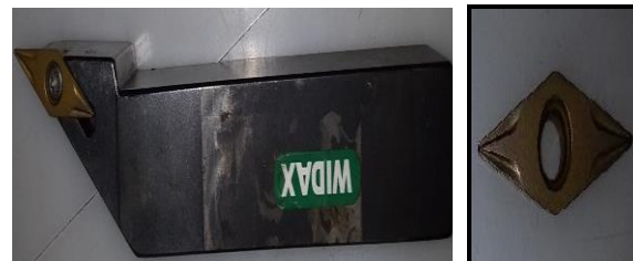
Figure2 Turning tool and Insert
