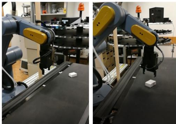
Fig. 11. Object being transported from the beginning of the conveyor (left picture) and the anthropomorphic robot executing the movement to pick the object (right picture)
