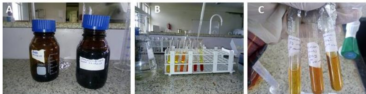
Figure 5: (A) DNSA reagent (B) Standard curve samples of glucose (C) Testing samples of paper of 5, 10 and 20 gm paper biomass hydrolysate.
