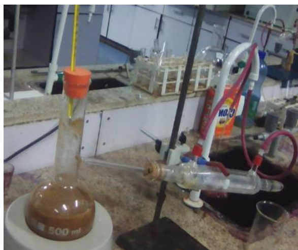
Figure 8: Simple Distillation setup
