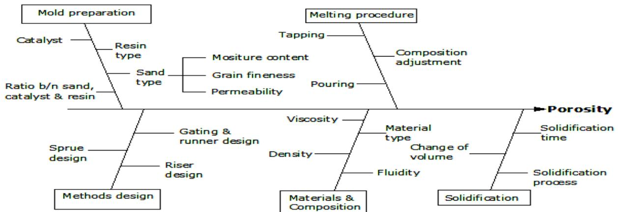
Fig.9Cause and effect diagram of porosity
