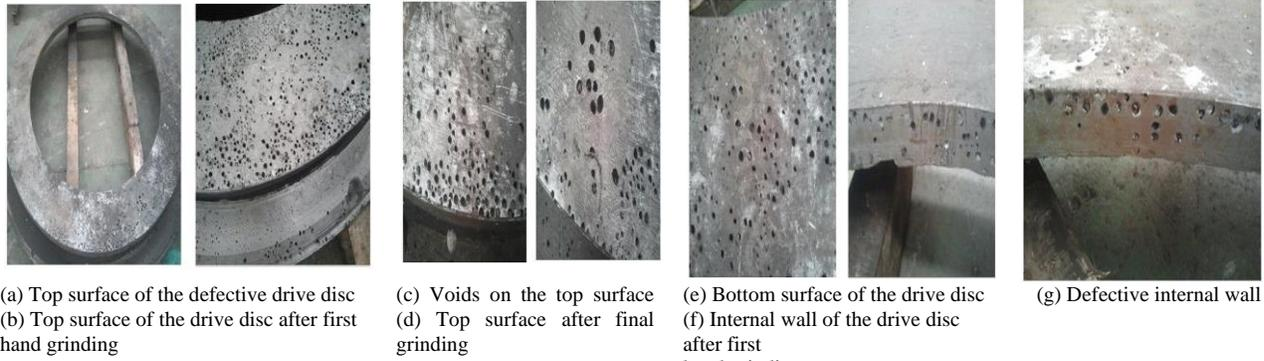
**Fig.2. Defective drive disc component**
