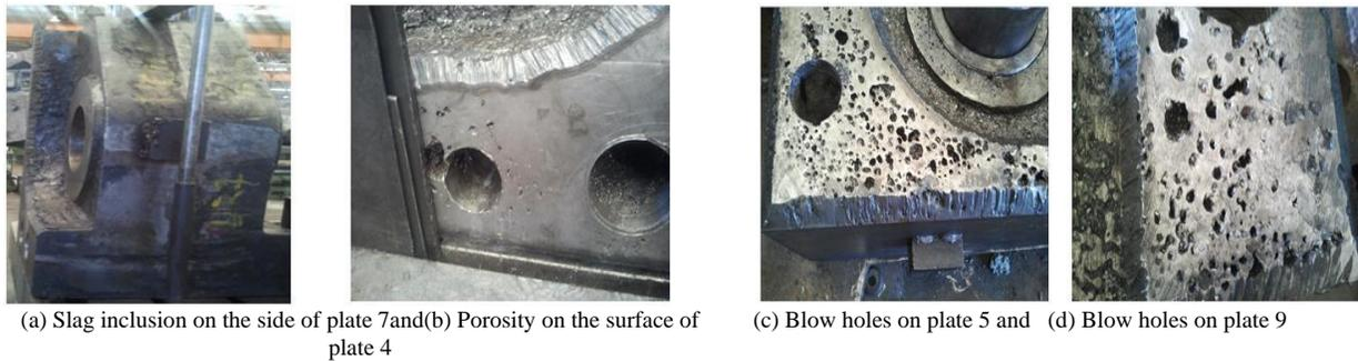
**Fig. 3. Defective headstock component**
