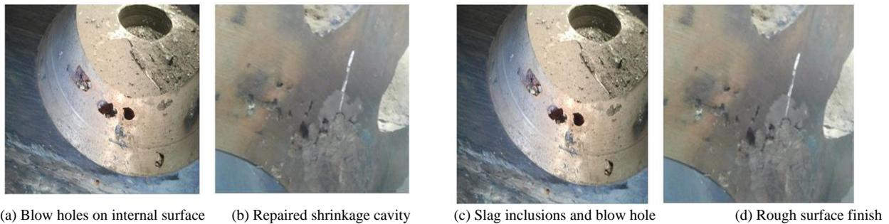
**Fig.4. Defective pinion gear component**
