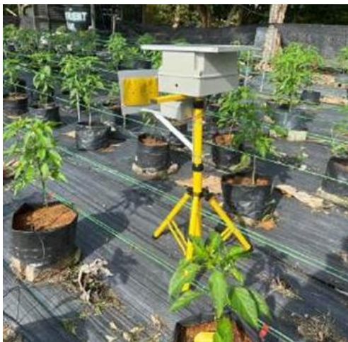
Fig. 7 Hardware setup for the IoT-based pest detection system
