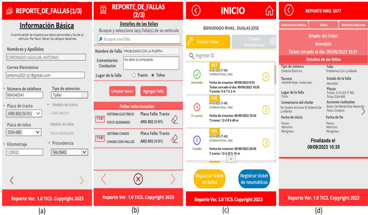
Fig. 4 Sprint backlog 1: User driver. (a) create fault reports, (b) prototype details of the report, (c) prototype report of malfunctions, and (d) prototype summary of the generated report.
