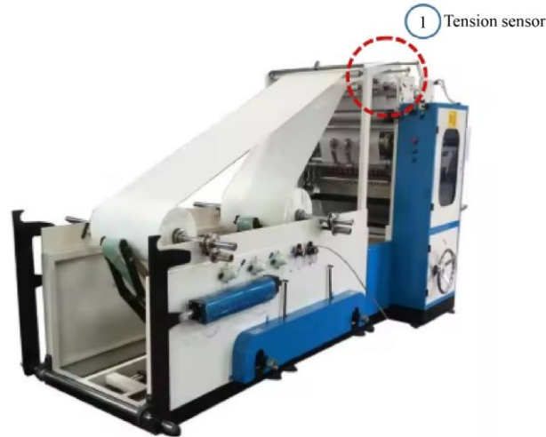
Fig. 2 Sensor Deployment Zone 1
