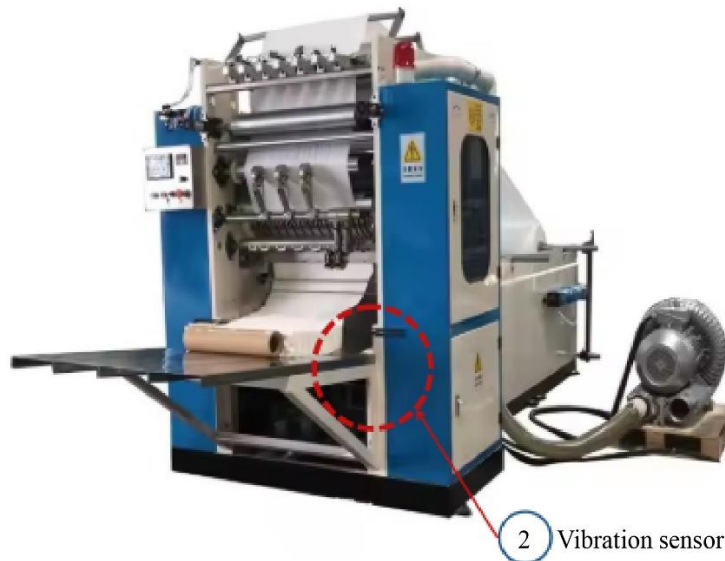
Fig. 3 Sensor Deployment Zone 2
