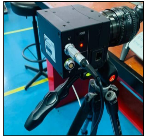
Fig. 4 High-speed video camera set-up for digital imaging measurements
