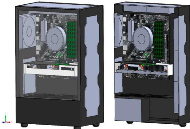
Fig. 2 Assembly used for simulations with the XPG VALOR AIR case
