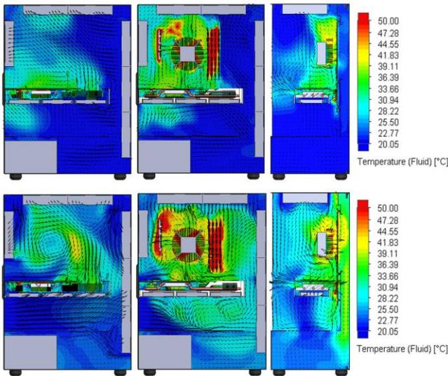
**Fig. 8 Air temperature contours with six case fans**
