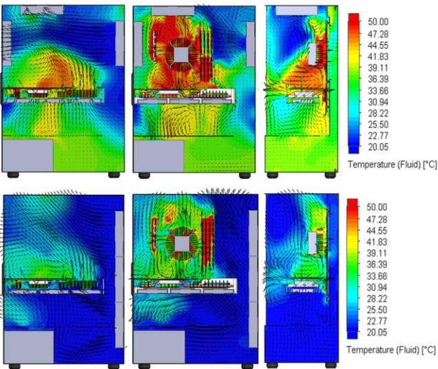
**Fig. 9 Air temperature contours with three case fans**
