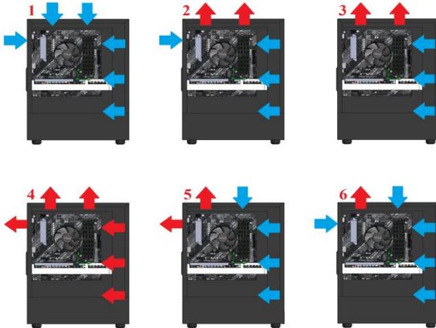
Fig. 3 Configurations used in the simulations with six fans in the XPG VALOR AIR case
