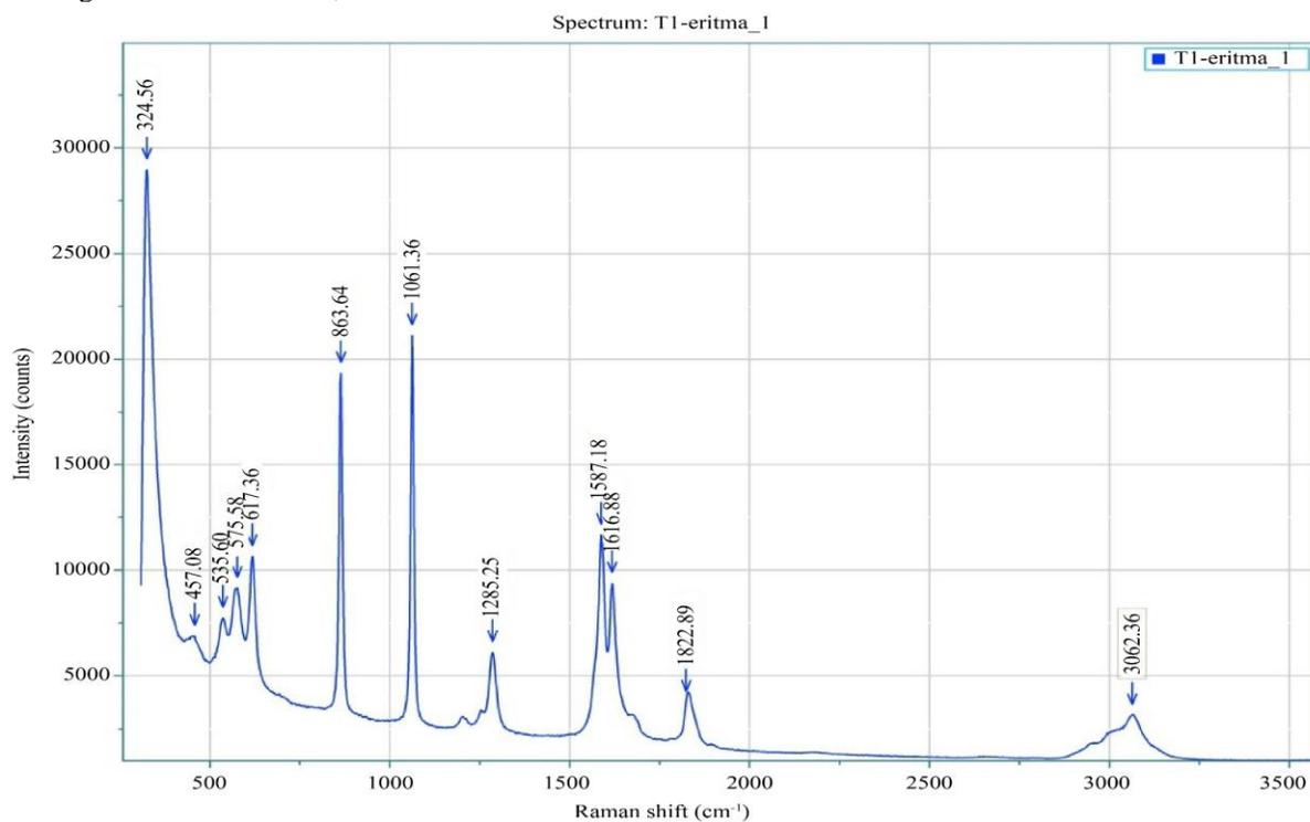
Fig. 8 Raman spectrum of the resulting terephthalamide
