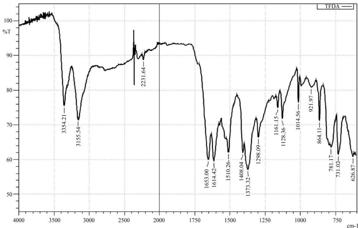
Fig. 7 IR spectrum of the resulting terephthalamide
