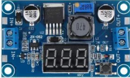
Fig. 13 LM2596 voltage regulator
