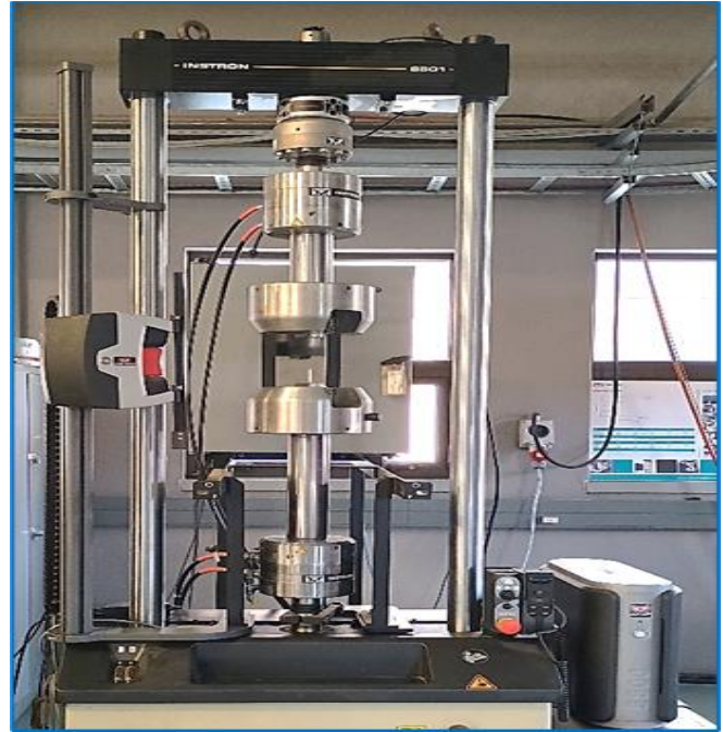
Fig. 3 100kN Instron 8801 servo hydraulic fatigue testing machine
