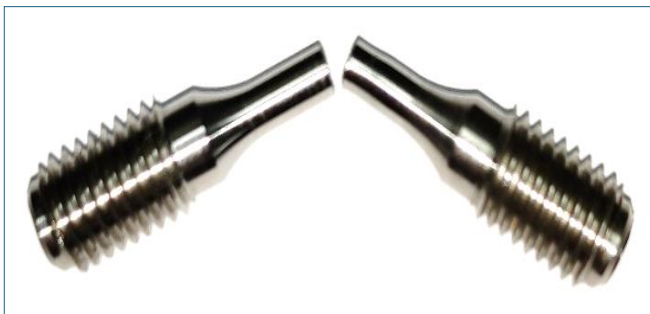
Fig. 10 Specimen of the confirmation experiment after fatigue failure
