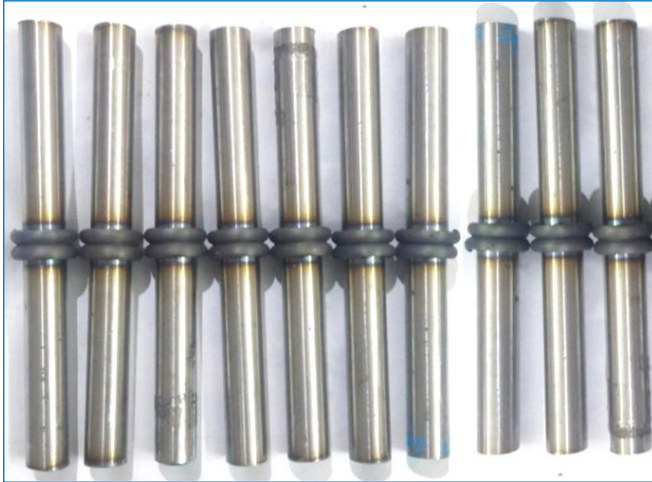
Fig. 2 AISI 316L friction welded to AISI 316L
