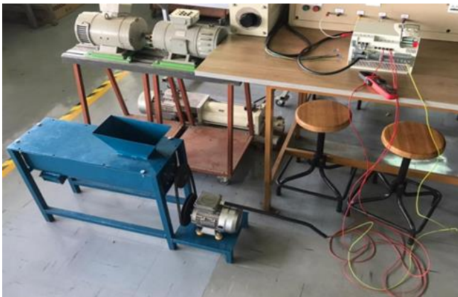
Fig. 3 A pictorial view of the fabricated dehulling machine connected to a variable speed drive (VSD)
