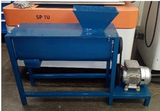
Fig. 2 A pictorial view of the fabricated dehulling machine
