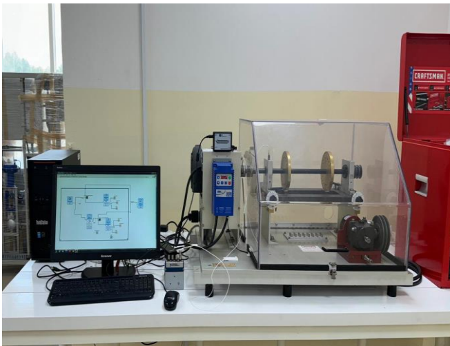
Fig. 2 Integration of MFS with LabVIEW software
