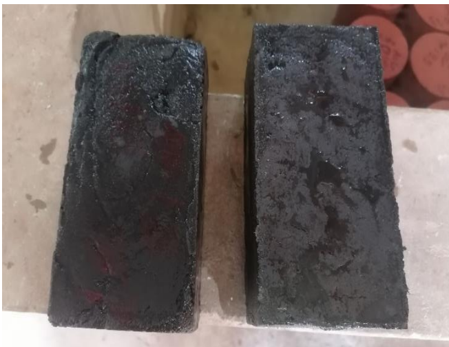
Fig. 13 Pavers after immersion for 3 days
