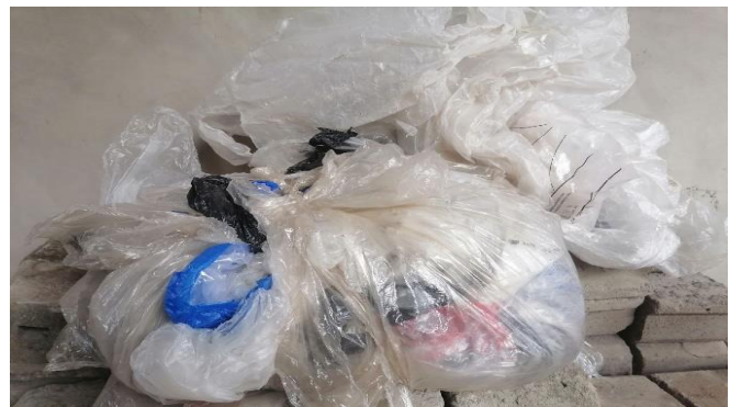
Fig. 1 Waste used for the manufacture of paving stones
