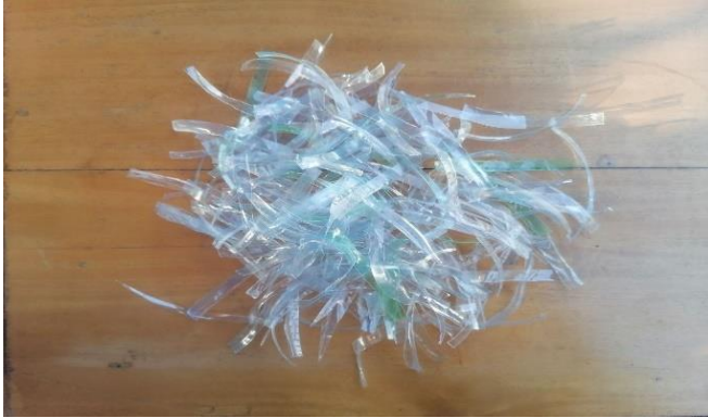
Fig. 3 Fibers obtained from plastic bottles
