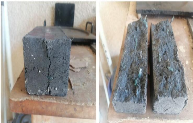
Fig. 11 Appearance of improved pavers after tensile failure
