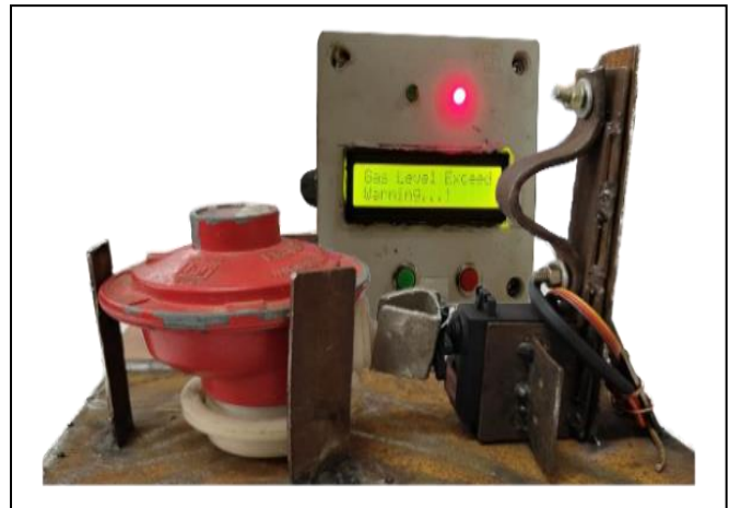
Fig. 9 Leakage controlling system
