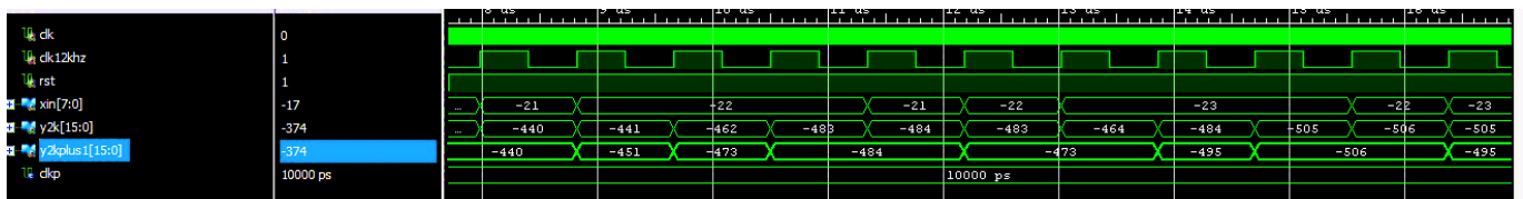
Fig. 17 Simulated output waveform for 2-parallel 4-tap FIR filter
