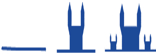
Fig. 1 Construction of Fractal curve (a) Straight line (b) Straight line with two hexagon-like head structures (c) Proposed 15-Segment fractal curve
