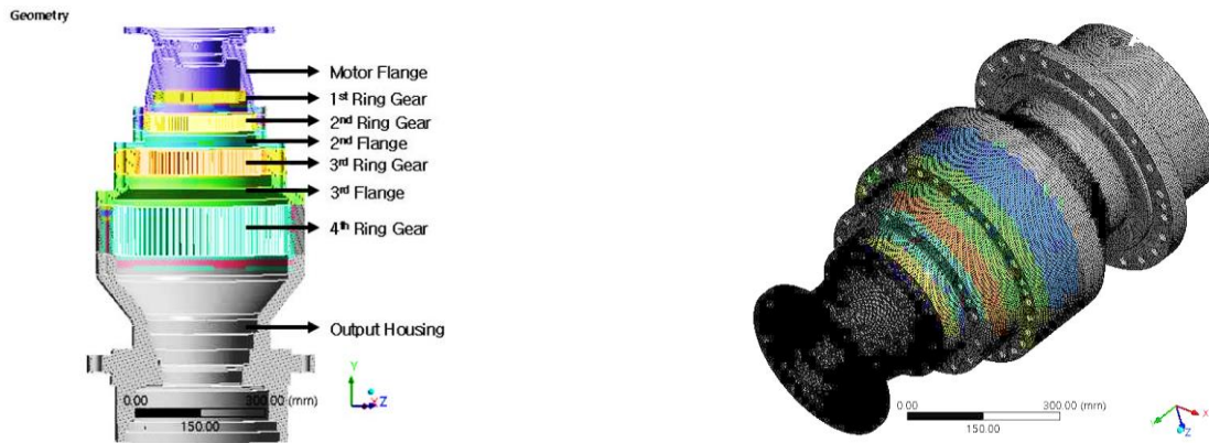
Fig. 1 Finite element analysis model of yaw gearbox housing for wind turbines
