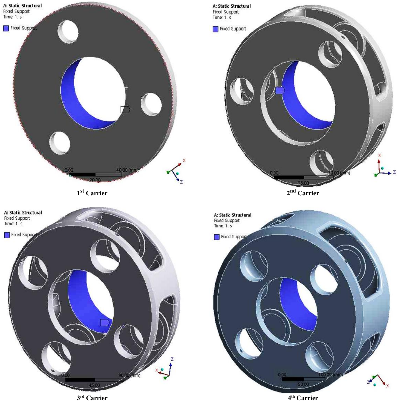
Fig. 6 Boundary conditions of yaw gearbox carriers
