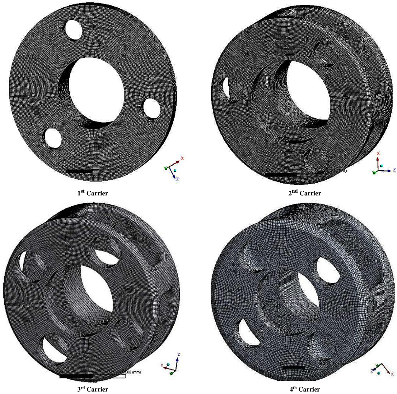
Fig. 5 Finite element analysis model of yaw gearbox carriers
