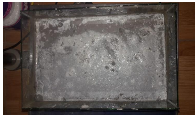
Fig. 6 Disposal of paste tailings with cement in the last layer - Design 3
