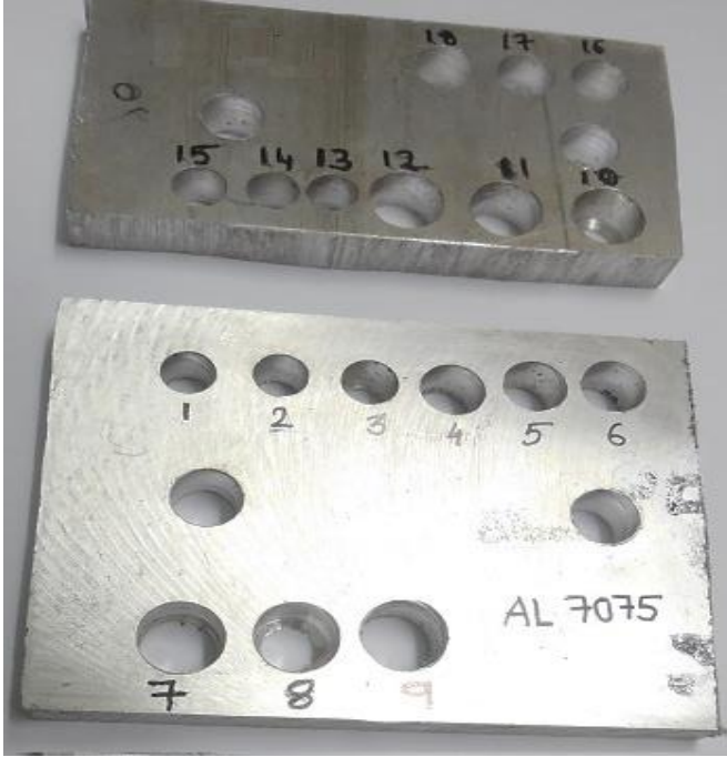
Fig. 5(c) Samples of AA7075 alloy workpieces after drilling
