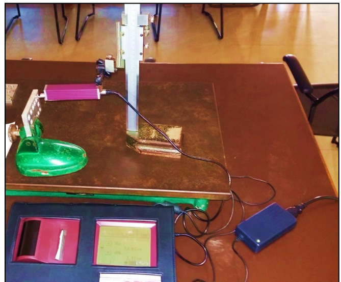
Fig. 5 (b) Surface roughness measurement apparatus
