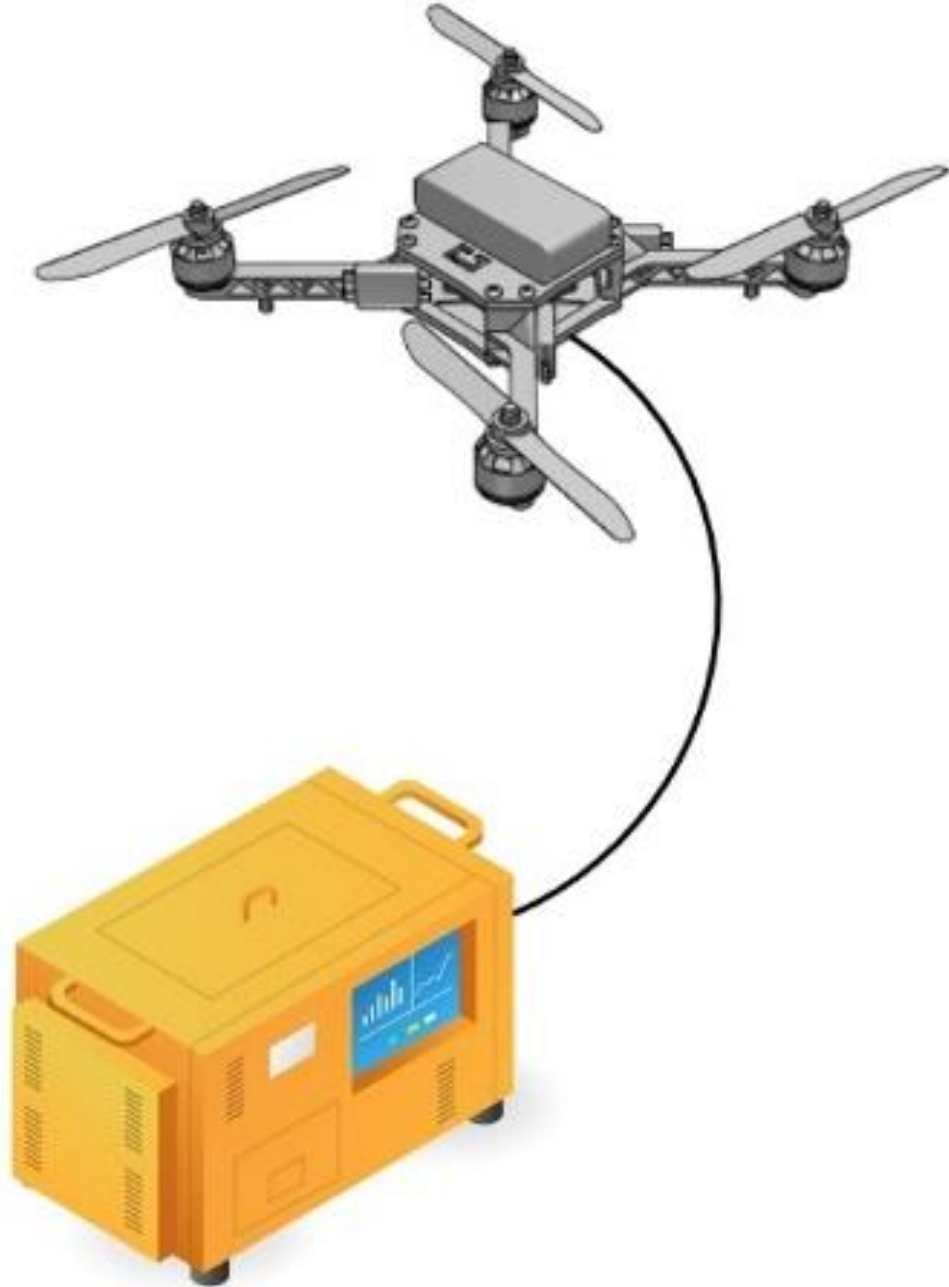
Fig. 1 Tethered drone system
