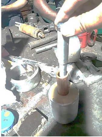
Fig. 1 Experimental set-up showing copper tube and cylindrical channel
