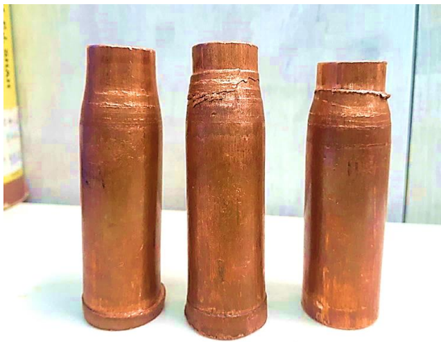
Fig. 2 Original copper tube and TCTP processed samples
