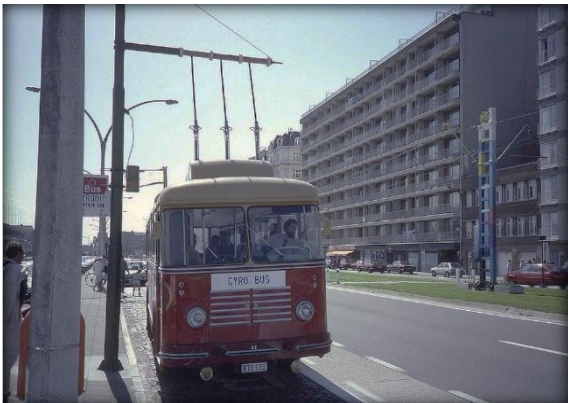
Fig. 2 Flywheel powered Gyro Bus [35]
