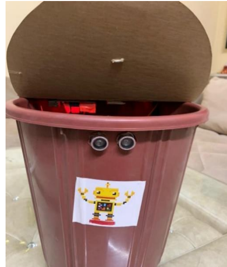
Fig. 8 Lid open when a human is near the dustbin
