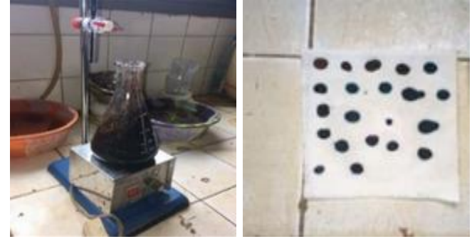
Fig. 5 Some steps for performing the methylene blue test.
