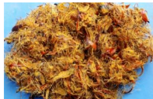
Fig. 9 Photo of palm fibers after oil extraction
