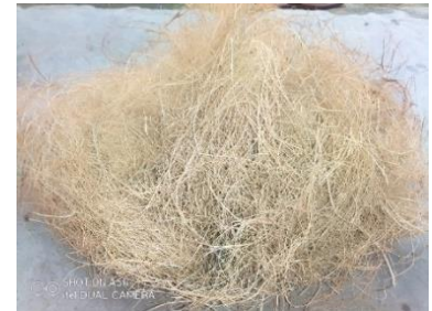
Fig. 8 Photo of the coconut fibers after treatment
