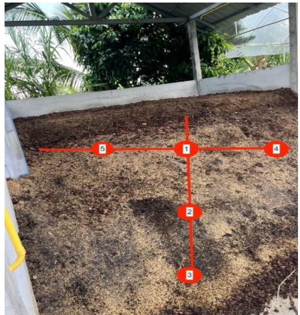
Fig. 4 The five sensor points in the composting plant
