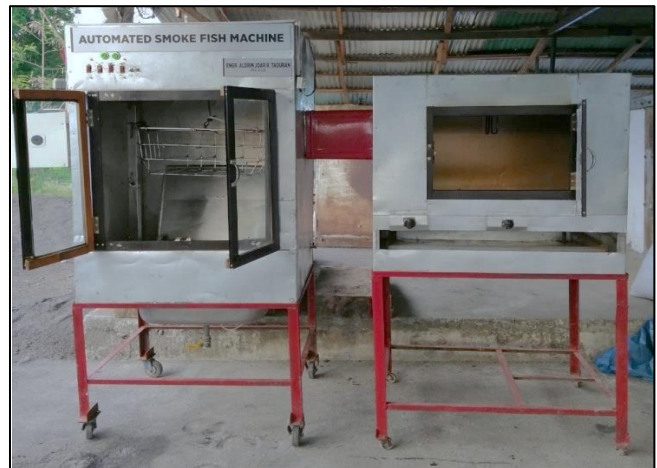
Fig. 12 Actual microcontroller-based smoked fish machine
