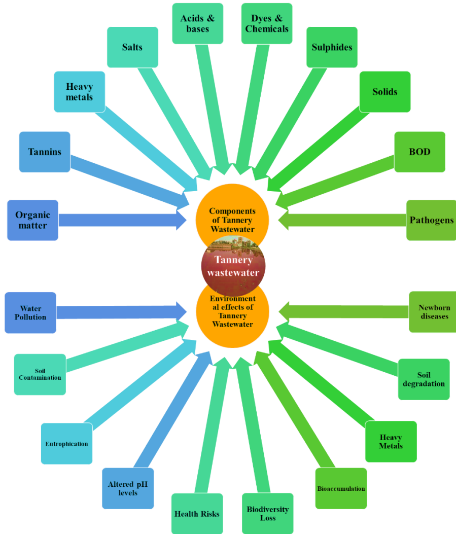
Fig. 1 Overview of components and environmental effects of tannery wastewater
