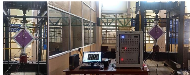
Fig. 13 (b) Experimental setup for RC frame
