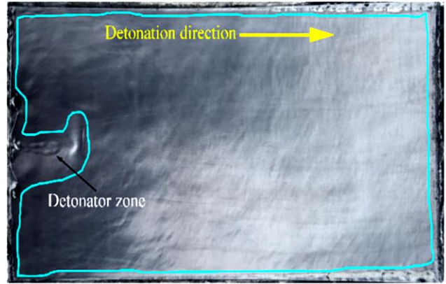
Fig. 7 Photograph of the recovered Ta/Fe sample after explosive welding
