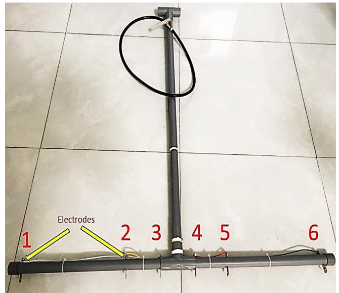
Fig. 4 Electrode for measurement soil EC in paddy field
