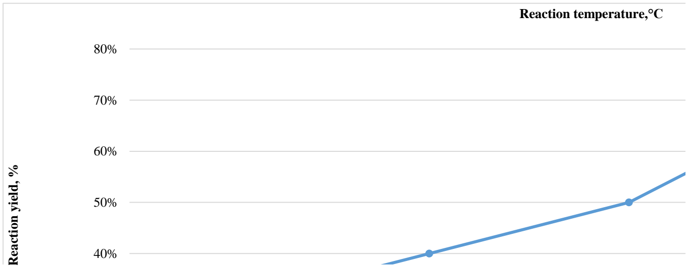
Fig. 2 The effect of temperature on the efficiency of the reaction during the synthesis of PANS raw material
